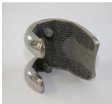
Femoral (knee) implant with designed porosity - © Econolyst
