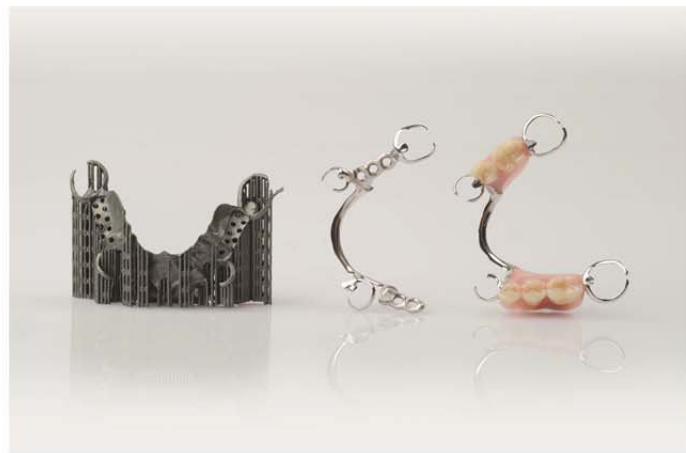
Partial denture manufactured using EOS Direct Metal Laser sintering © EOS
