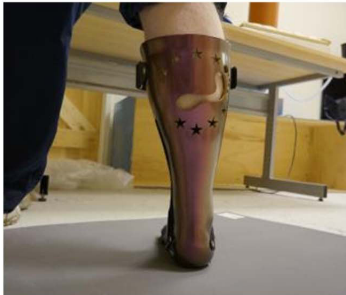
Rigid full foot orthosis produced by selective laser sintering from patient scan data - © Peacock Orthotics Ltd
