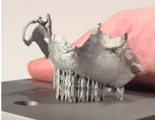
Bespoke mandible (jaw) reconstruction made using Selective Laser Melting © Econolyst
