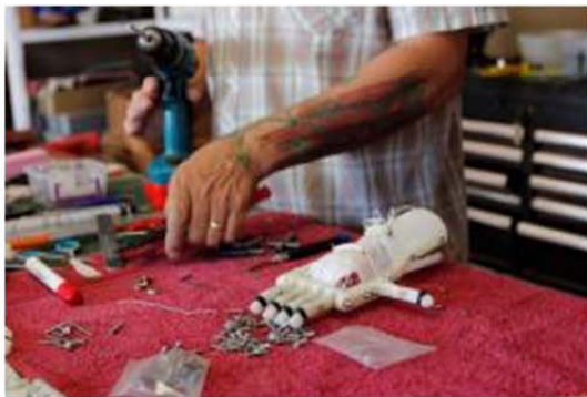
3D printed Robohand downloaded from Thingiverse for local manufacture & assembly - © Makerbot
