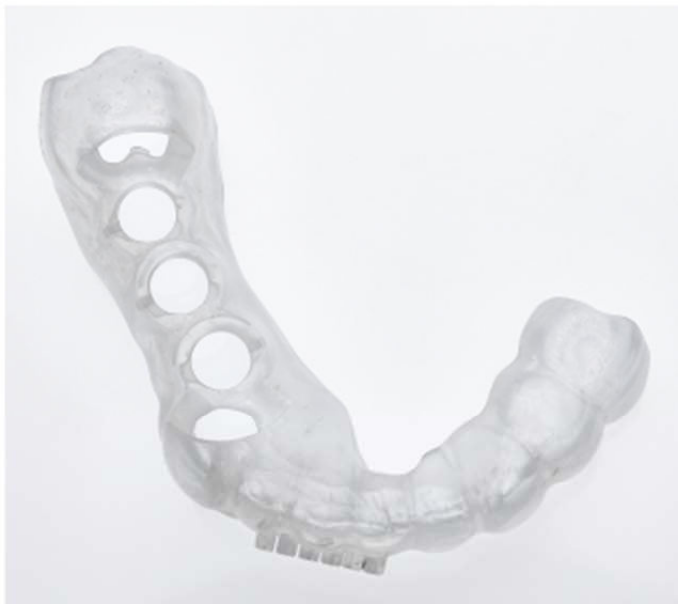
Dental surgical drilling guide produced using a resin base ALM platform © Envisiontec
