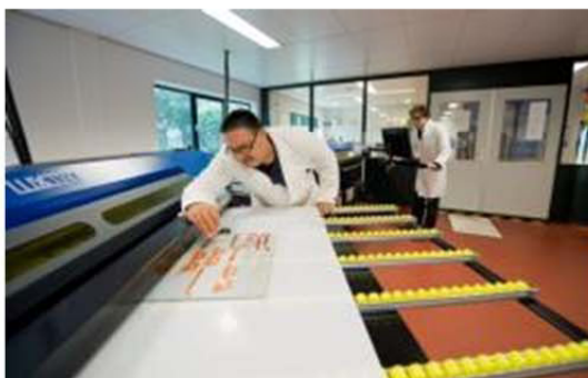
Additive Manufacturing of 'Spectacles' with integral frames and prescription lenses - © Luxexcel
