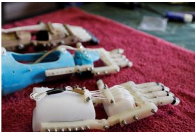
Robohand — consumer 3D printed, open source prosthetic for sub $100 © Makerbot
