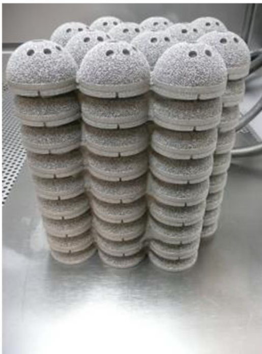
Production batch of 108 acetabula cup (hip socket) implants produced in 95-hours © Arcam AB
