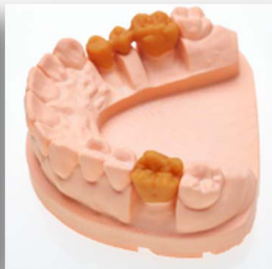
Step 2 – produce castable 3D printed crowns and bridge from 3D CAD data © Envisiontec
