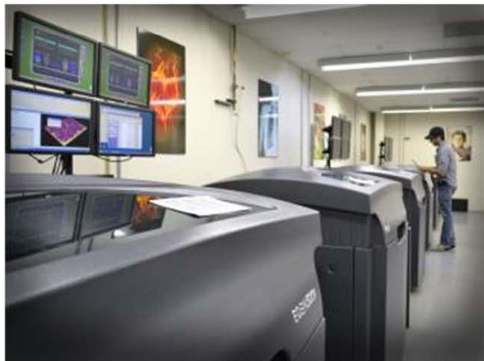
The ClearCorrect production facility using Objet Eden 500V printers - © Clear Correct
