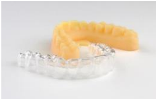
A vacuum formed dental aligner shown next to a bespoke vacuum forming tool made using the Stratasys Polyjet process - © ClearCorrect
