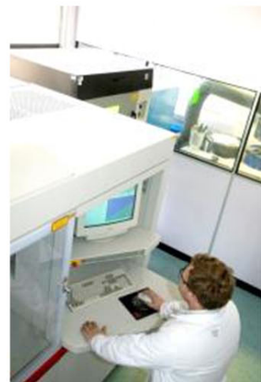
3D Systems Stereolithography machine used for polymeric additive layer manufacturing using photocurable monomers- © Econolyst
