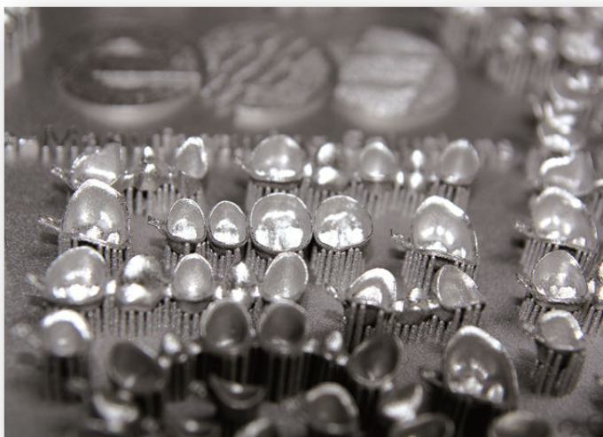
Full platform of dental caps and crowns produced using the EOS Direct Metal Laser Sintering process © EOS
