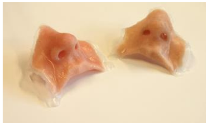
Soft Tissue Prosthesis noses manufactured using modified Z-Corp 3D Printing process - © Fripp Design Ltd
