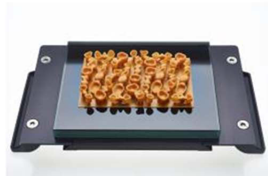
A platform of dental crown and bridge patterns made in photocurable polymer prior to investment casting – © Envisiontec
