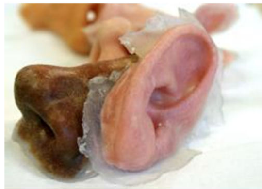
3D printed facial prosthetics manufactured using 3D scan data and sampling of the patients own skin tones - © Fripp Design Ltd
